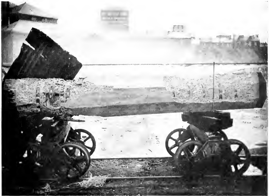
Column No. 4, after Test
