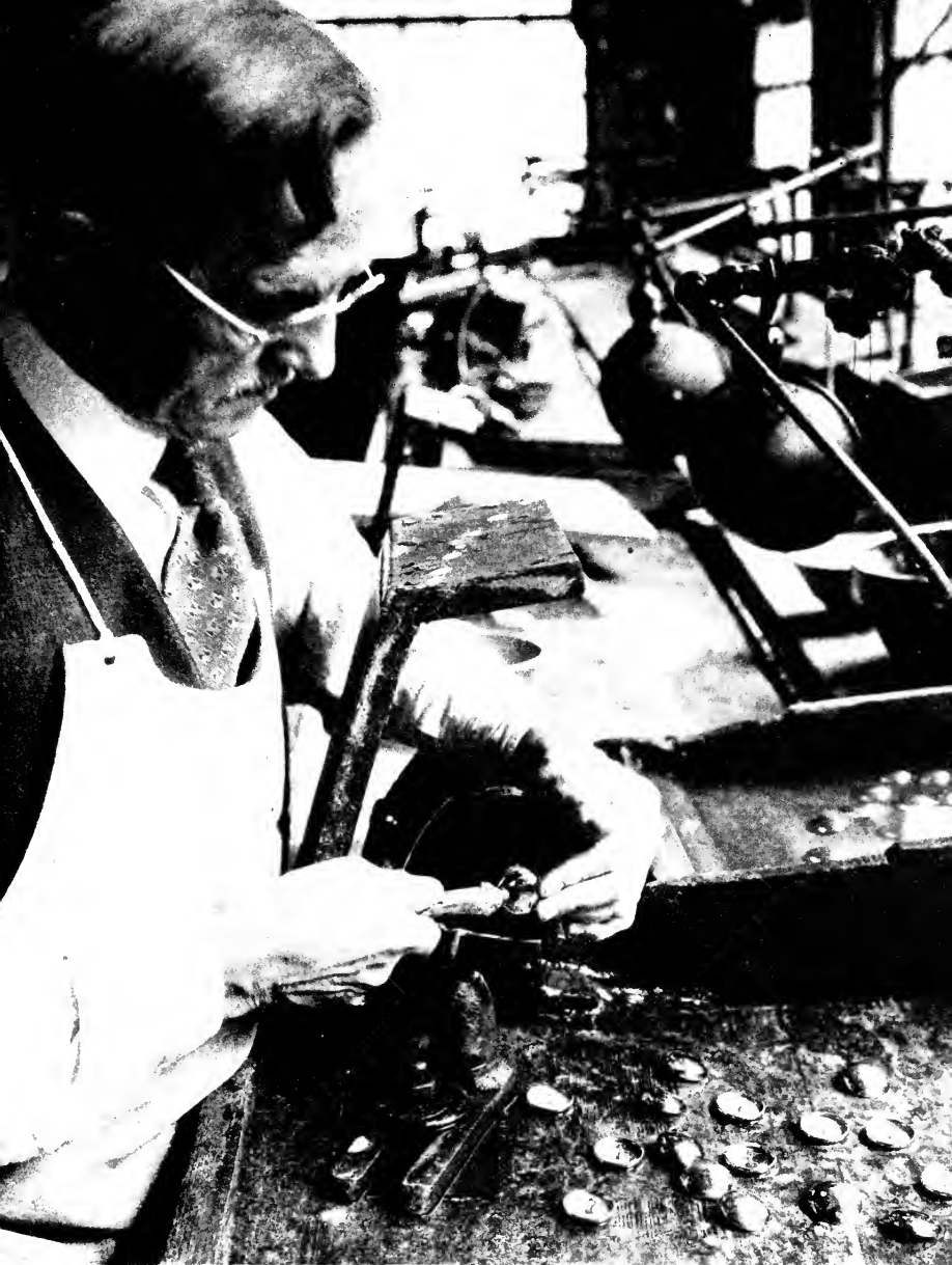
BURNISHING BRASS, SCOVILL MANUFACTURING COMPANY, WATERBURY
