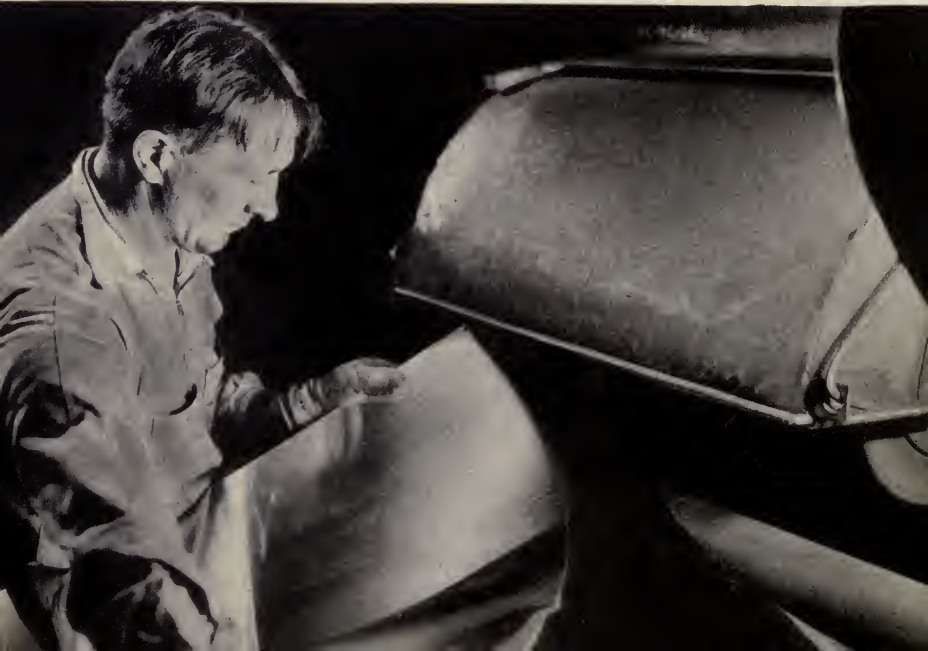
INSPECTING POLISHED COPPER SHEETS, AMERICAN BRASS COMPANY, ANSONIA
