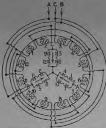
FIG. 60.—Showing the diagram Fig. 59 reconnected from series to parallel star.
