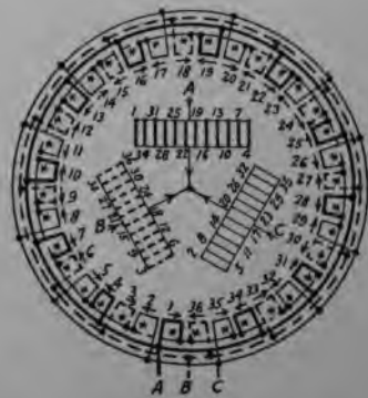
FIG. 252.—Twelve pole, three phase, twelve parallel star.
