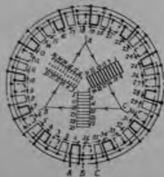
FIG. 258.—Twelve pole, three phase, twelve parallel delta.
