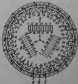
FIG. 252.—Twelve pole, three phase, twelve parallel star.
