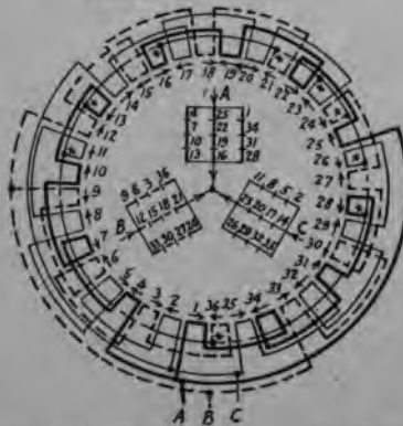
FIG. 249.—Twelve pole, three phase, three parallel star.
