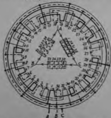
FIG. 255.—Twelve pole, three phase, three parallel delta.
