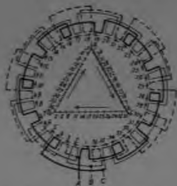
FIG. 253.—Twelve pole, three phase, series delta.
