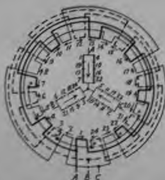
FIG. 222.—Eight pole, three phase, two parallel star.
