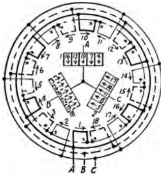
FIG. 212.—Six pole, three phase, six parallel star.
