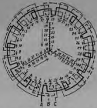
FIG. 247.—Twelve pole, three phase, series star.
