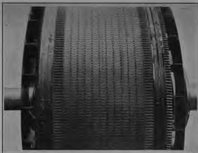
FIG. 33.—Rotor with slots as in Fig. 21 wound with strap coils of the "wave" type.
