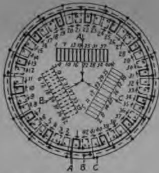
FIG. 266.—Fourteen pole, three phase, fourteen parallel star.
