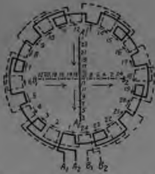
FIG. 241.—Twelve pole, two phase, series.
