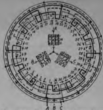
FIG. 250.—Twelve pole, three phase, four parallel star.
