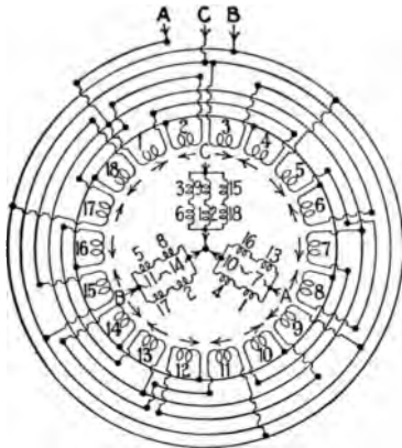
FIG. 62.—Three-phase, six-pole winding connected three parallel star.
