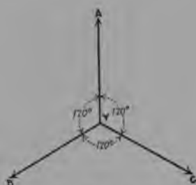
FIG. 172.—Normal winding relation.
