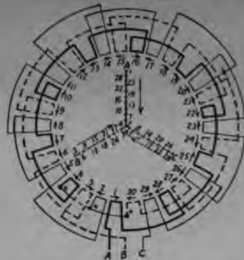
FIG. 233.—Ten pole, three phase, series star.
