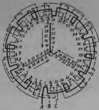
FIG. 247.—Twelve pole, three phase, series star.
