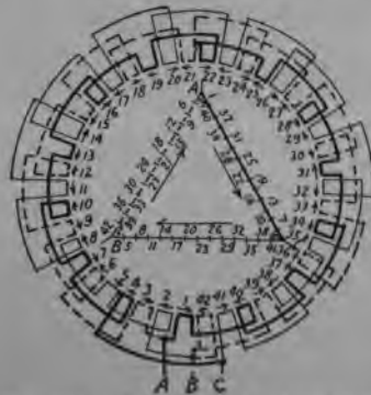
FIG. 267.—Fourteen pole, three phase, series delta.
