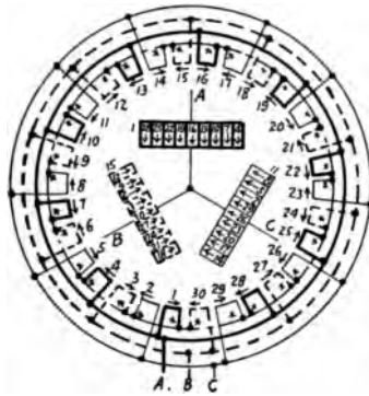
FIG. 236.—Ten pole, three phase, ten parallel star.
