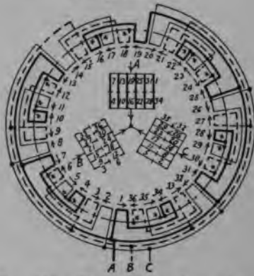
FIG. 251.—Twelve pole, three phase, six parallel star.
