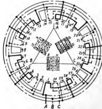
FIG. 239.—Ten pole, three phase, five parallel delta.
