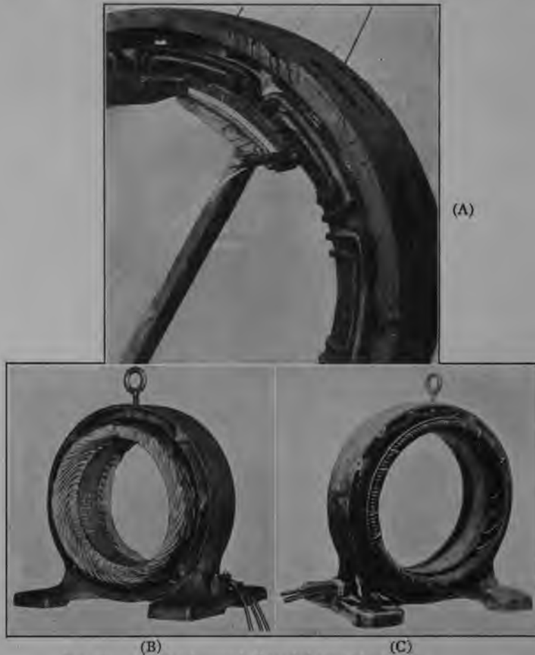
FIG. 27.—(A) Hand-wound, threaded type of winding. FIG. 28.—(B) "Fed-in" type—"mush coil" or one coil per slot. FIG. 29.—(C) "Fed-in" type—"diamond" or two coils per slot. Stators with partly closed slots.
