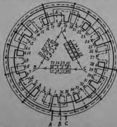
FIG. 255.—Twelve pole, three phase, three parallel delta.
