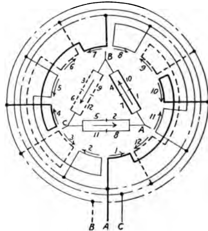
FIG. 203.—Four pole, three phase, two parallel delta.
