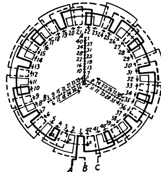
FIG. 263.—Fourteen pole, three phase, series star.
