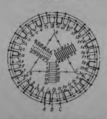
FIG. 258.—Twelve pole, three phase, twelve parallel delta.
