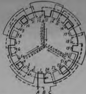
FIG. 221.—Eight pole, three phase, series star.
