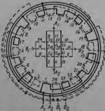
FIG. 243.—Twelve pole, two phase, three parallel.
