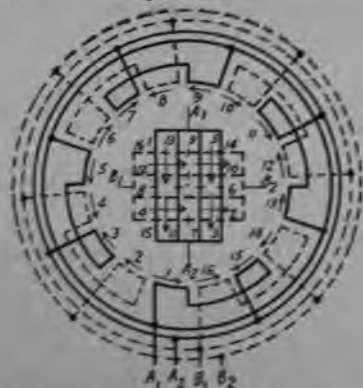
FIG. 219.—Eight pole, two phase, four parallel.
