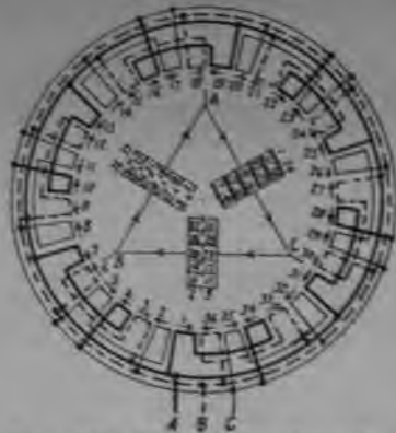
FIG. 257.—Twelve pole, three phase, six parallel delta.
