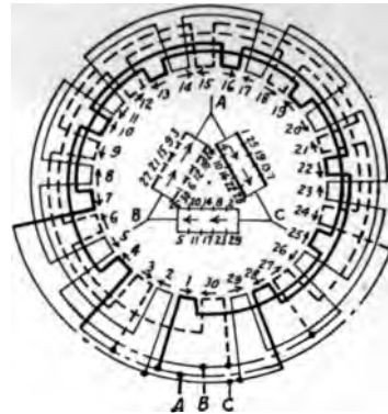
FIG. 238.—Ten pole, three phase, two parallel delta.
