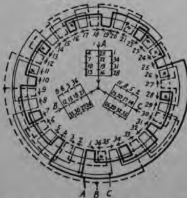
FIG. 249.—Twelve pole, three phase, three parallel star.
