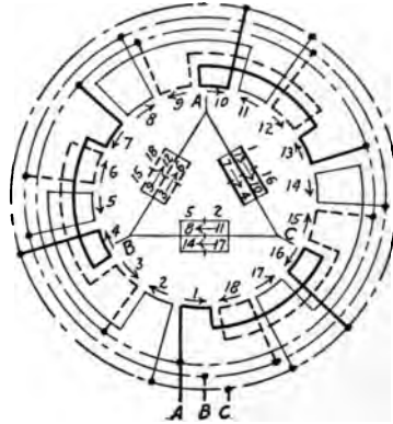
FIG. 215.—Six pole, three phase, three parallel delta.
