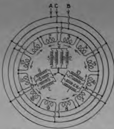
FIG. 61.—Showing the diagrams of Figs. 59 and 60 reconnected to four parallel star.
