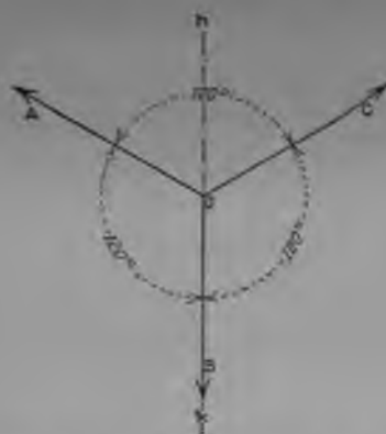
FIG. 86.—Normal relation of the currents in a three-phase motor.
