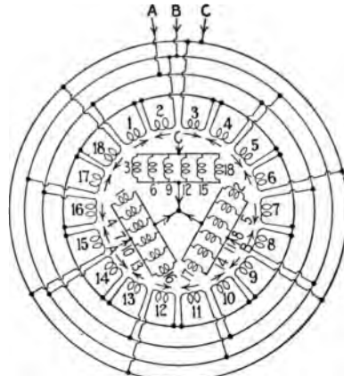
FIG. 63.—Three-phase, six-pole winding connected six parallel star.
