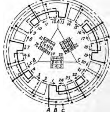
FIG. 227.—Eight pole, three phase, four parallel delta.
