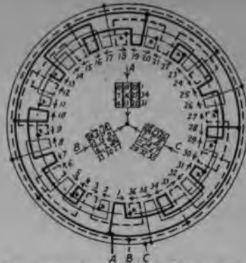
FIG. 250.—Twelve pole, three phase, four parallel star.
