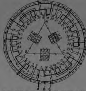
FIG. 256.—Twelve pole, three phase, four parallel delta.
