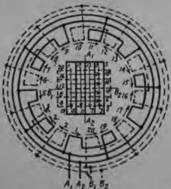
FIG. 231.—Ten pole, two phase, five parallel.
