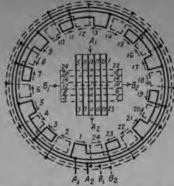
FIG. 245.—Twelve pole, two phase, six parallel.
