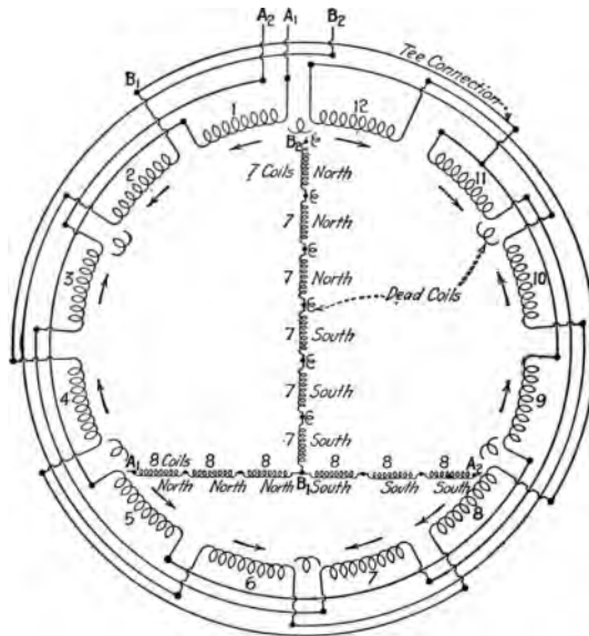
FIG. 120.—Preferable connection to Fig. 117 so-called "top to top" connection.
