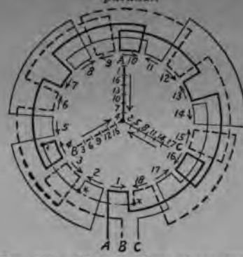
FIG. 209.—Six pole, three phase, series star.
