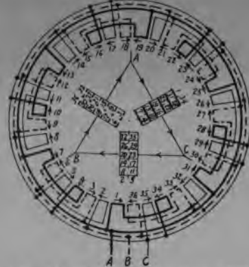
FIG. 257.—Twelve pole, three phase six parallel delta.
