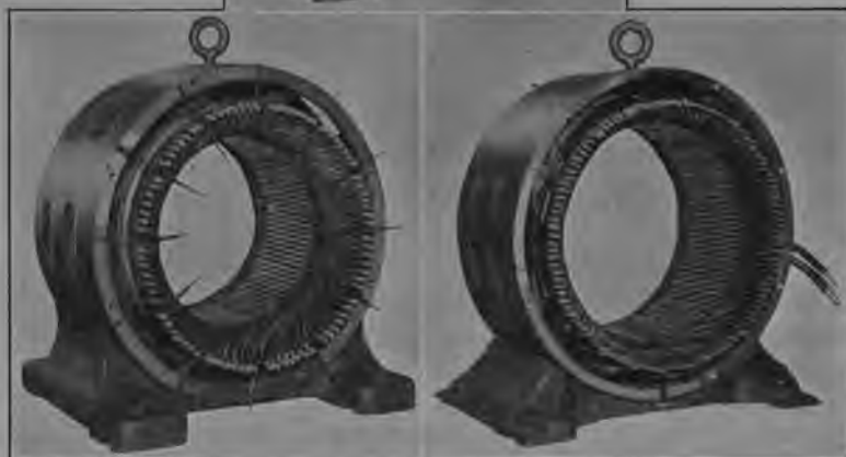
FIG. 166.—Coils connected into pole phase groups.
