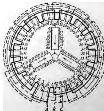
FIG. 264.—Fourteen pole, three phase, two parallel star.
