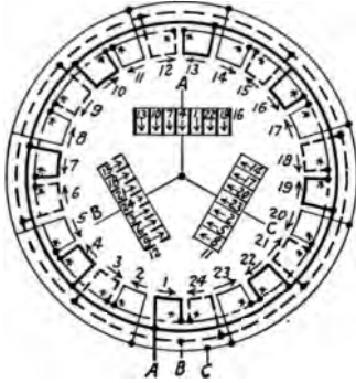
FIG. 224.—Eight pole, three phase, eight parallel star.
