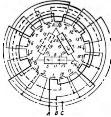
FIG. 214.—Six pole, three phase, two parallel delta.
