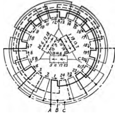
FIG. 226.—Eight pole, three phase, two parallel delta.
