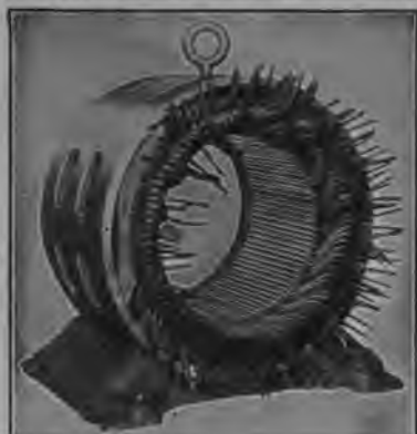
FIG. 271.—Coils wound but unconnected.
