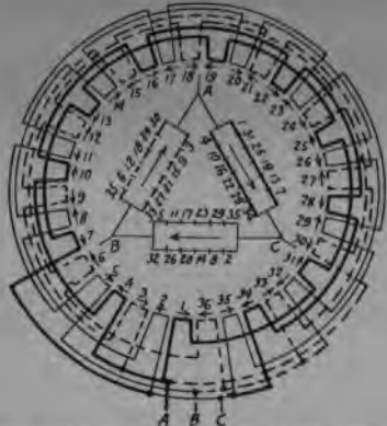
FIG. 254.—Twelve pole, three phase, two parallel delta.
