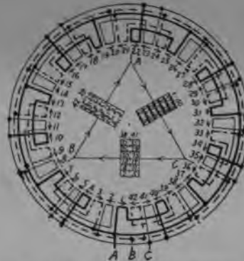
FIG. 269.—Fourteen pole, three phase, seven parallel delta.
