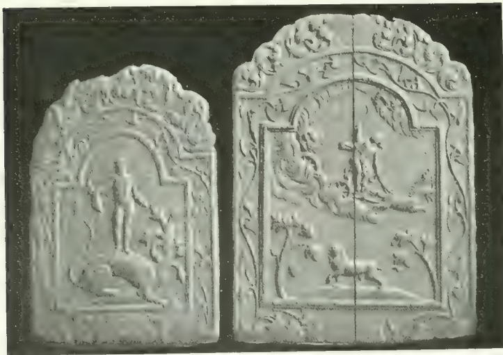
ORIGINAL WOODEN PATTERNS FROM WHICH FIREBACKS WERE MADE, AT ASHBURNHAM, SUSSEX
