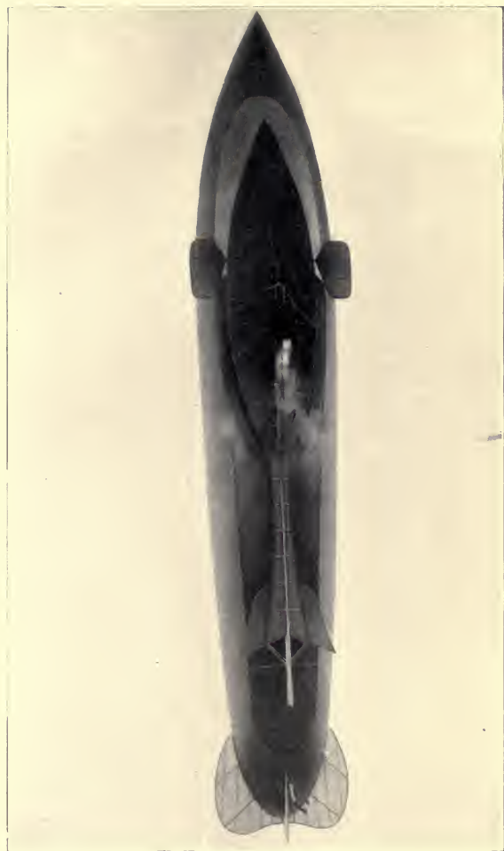
THE DIRIGIBLE "PATRIE" SEEN FROM BELOW, THE HORIZONTAL STABILISING EMPENNAGE CAN BE DISTINGUISHED AS WELL AS THE ELEVATING RUDDER IN FRONT
