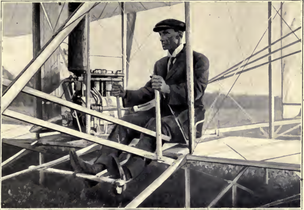
WILBUR WRIGHT AT THE HELM OF HIS AEROPLANE (THE TWO STEERING LEVERS MAY BE DISTINCTLY SEEN)
