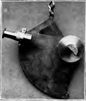
THE JOANNETON APPARATUS FOR RECORDING THE SPEED OF AIRSHIPS
