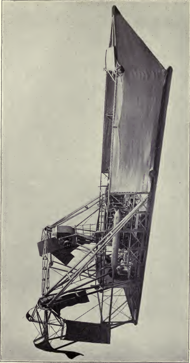
THE CAR OF THE "PARSEVAL," Showing blades of propellers, which fold over when at rest
