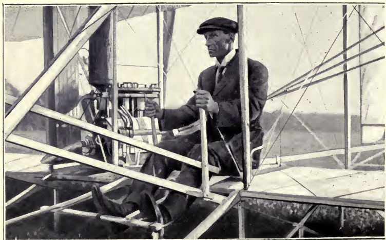
WILBUR WRIGHT AT THE WHEEL OF HIS AEROPLANE SHOWING THE TWO CONTROL LEVERS
