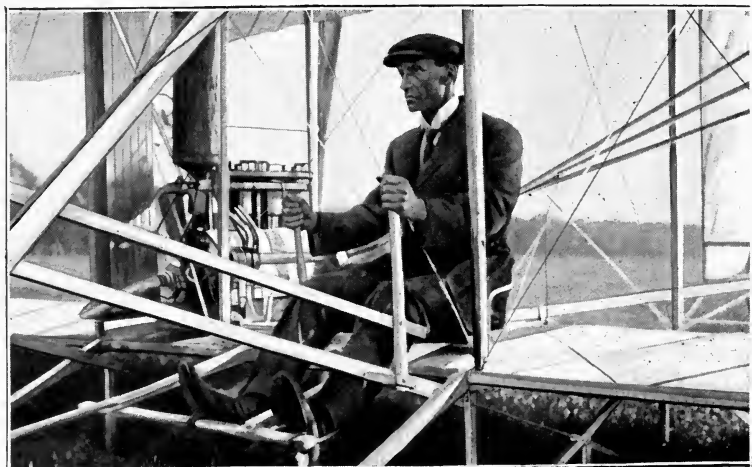
WILBUR WRIGHT AT THE WHEEL OF HIS AEROPLANE SHOWING THE TWO CONTROL LEVERS
