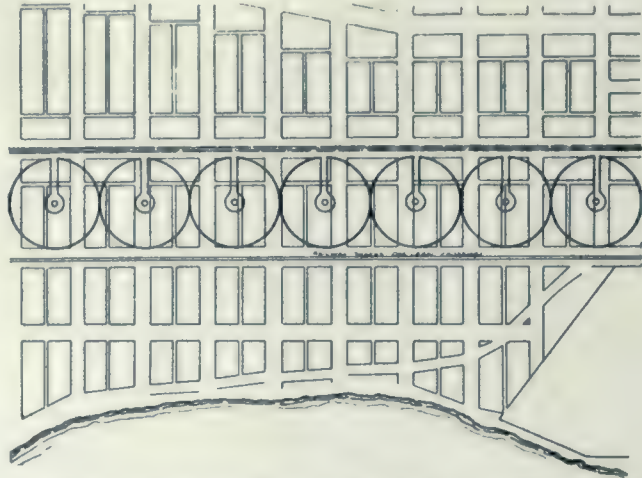
Fig. 1.—Plan showing how the circles in which the houses are grouped can be adapted to rectangular city blocks. This scheme, it is claimed, eliminates a number of common engineering difficulties and offers certain economical advantages as regards up keep and service.
