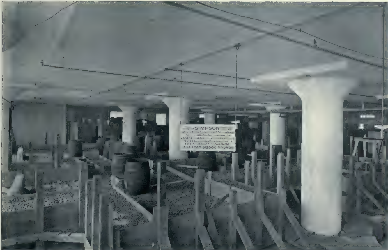
TEST OF FLOOR SLAB LOADED TO DOUBLE THE NOMINAL CAPACITY, THE ROBERT SIMPSON MAIL ORDER BUILDING, TORONTO.
