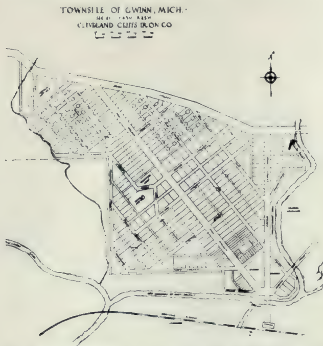
Fig. 6—Plan of a Portion of the Town Site of Gwinn, showing the Arrangement of the Semi-detached Houses Upon the Lots. Longer Views are Obtained Between Houses by Altering or Staggering the Houses on Either Side of the Street.
