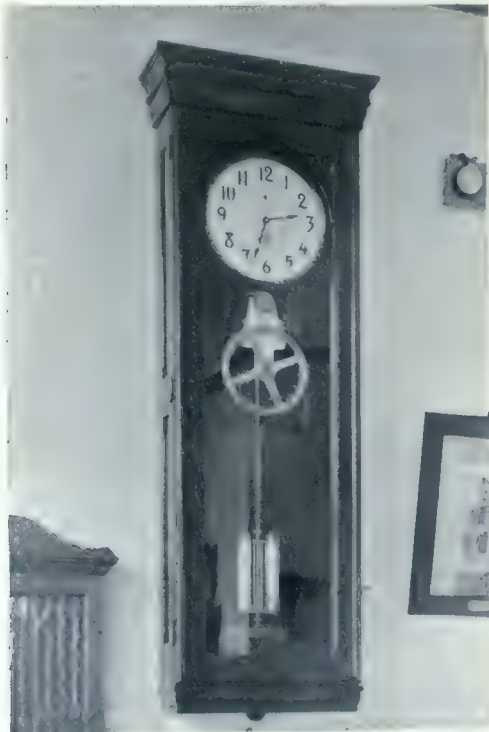
Type of Master Clock used in connection with Time Regulating System in London (Ont.) Technical and Art School.
