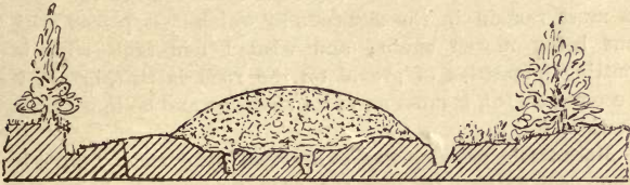
FIG. 3.—ENGLISH ROAD ABOUT 1809, Showing its state before and after repair. Well "barrelled!"
