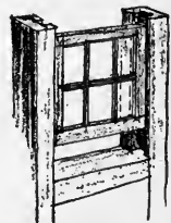
Crude beginning of the sliding Sash.
