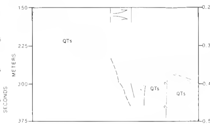
SLUMP boundaries solid where well defined, dashed where inferred, queried where uncertain. Arrows indicate direction of movement. Zone of movement extends to a subbottom depth of approximately 90 m in sediments of late Tertiary and Quaternary (QTs) age. Note apparent slip surfaces and back-rotated reflectors. Example from Uniboom profile across Ascension Canyon, central California continental margin.
