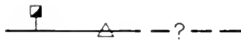
FAULT: solid where well defined, dashed where inferred, queried where uncertain. Bar and age symbol shown on downthrown side of fault that has seafloor expression. Fault displaces seafloor, offsetting sediments of presumed late Tertiary and Quaternary (QTs) age and juxtaposing subjacent units of Miocene (Tm) and possibly Pliocene (Tp?) ages. Also note inferred fault within probable Miocene section, and folded strata. Example from Uniboom profile across Tanner Bank, middle southern California continental borderland (after Greene and others, 1975, their Figure 3).
