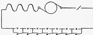
FIG. 127.—SERIES-WOUND GENERATOR WITH ARC LAMPS IN SERIES.
