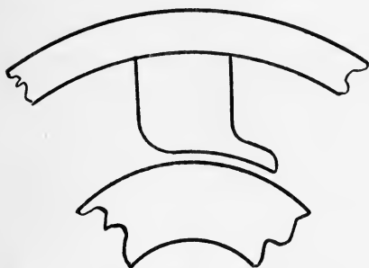
FIG. 8.—ARRANGEMENT OF TIP TO AVOID MAGNETIC JOINTS.
