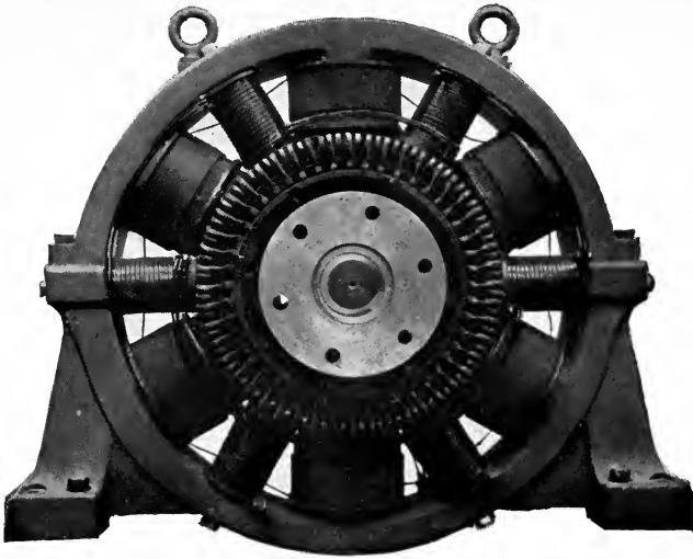
FIG. 59.—INTERPOLE MACHINE SHOWING EQUALIZER RINGS (PHENIX DYNAMO COMPANY).
