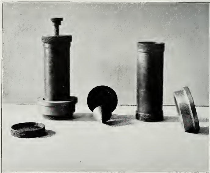
FIG. 1. Centrifuge cups, according to the design of Stansfield and Sutherland, for separating coal samples into fractions of different densities.
