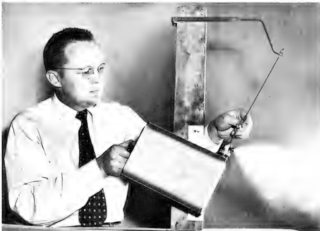
Z. & W. sprayer attached to garden-hose fitting soldered to gallon spray can.
