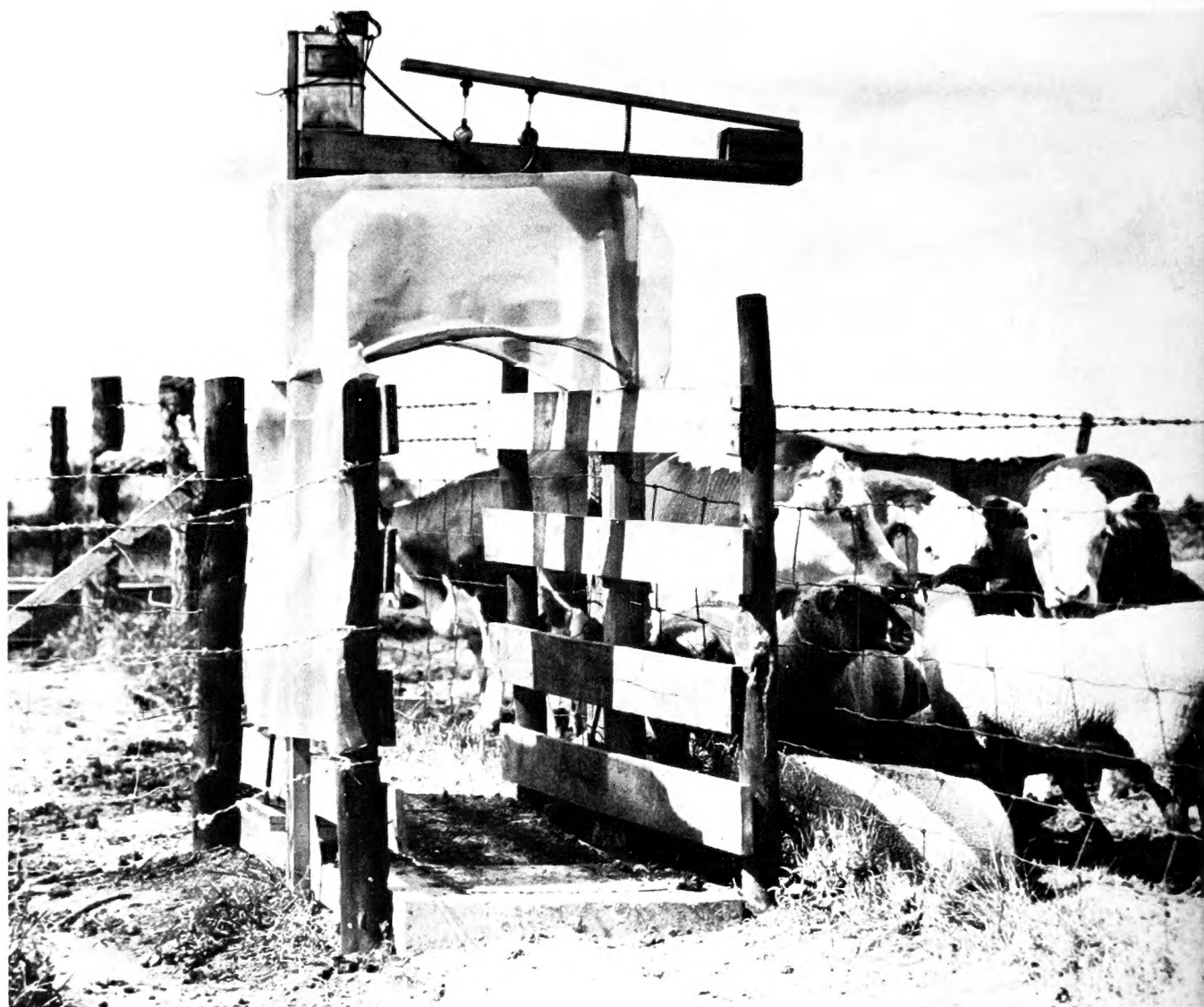
Automatic microspray applicator used in 1950 experiments for control of horse flies on beef cattle.
