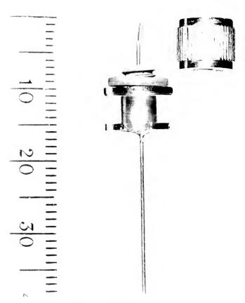
Fig. 8. Photograph of the cannula with inserted stilette (seen as bent wire protruding from upper end) and protective screw cap. Scale in mm.
