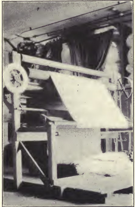
Figure 43. Perch for Inspecting Textile Fabrics—The Shelton Looms
