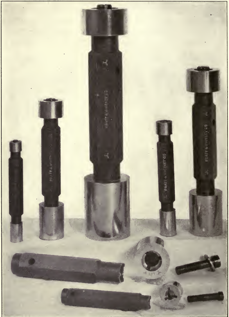
Figure 72. Adjustable Limit Plug Gages with Reversible Ends—Pratt and Whitney Type
