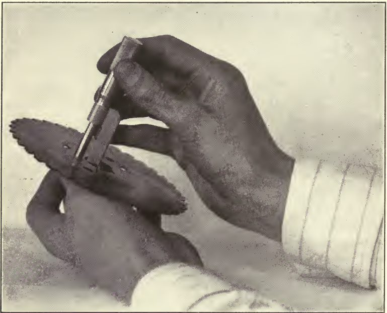
Figure 51. Method of Using Hub Micrometer Caliper #241—Brown and Sharpe Manufacturing Company
