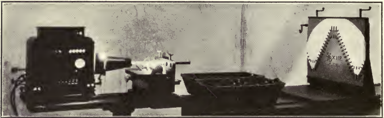
Figure 77. General View of Hartness Screw Thread Comparator
