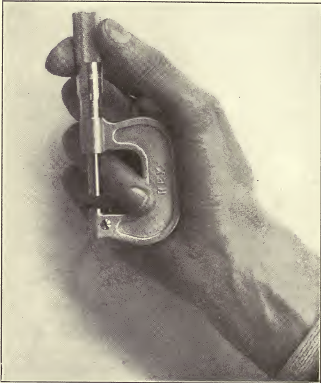
Figure 4. A Common Method of Holding a Micrometer Caliper Courtesy of Brown and Sharpe Manufacturing Company.
