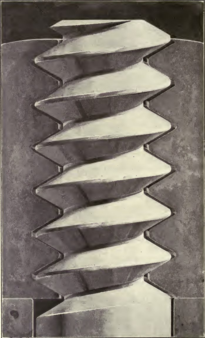
Figure 74. An Exaggerated Form of Stud
