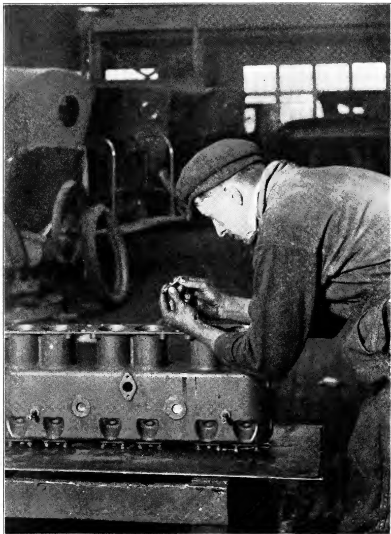
Figure 59. Reading Inside Micrometers after Measuring Inside of Cylinder Brown and Sharpe Manufacturing Company.
