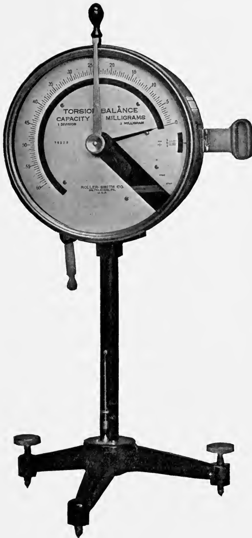
Figure 89. Precision Torsion Balance—Roller-Smith
