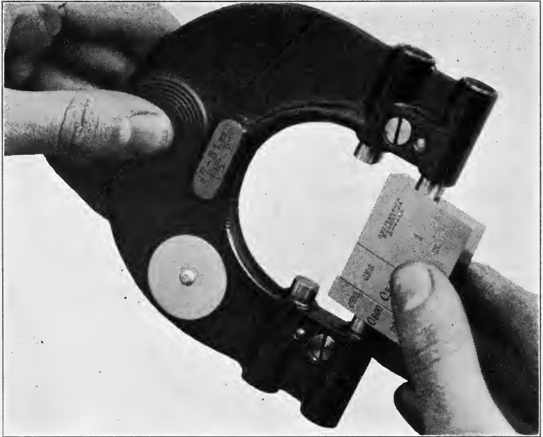
Figure 52. Setting a Johansson Adjustable Limit Snap Gage by Means of Johansson Gage Blocks
