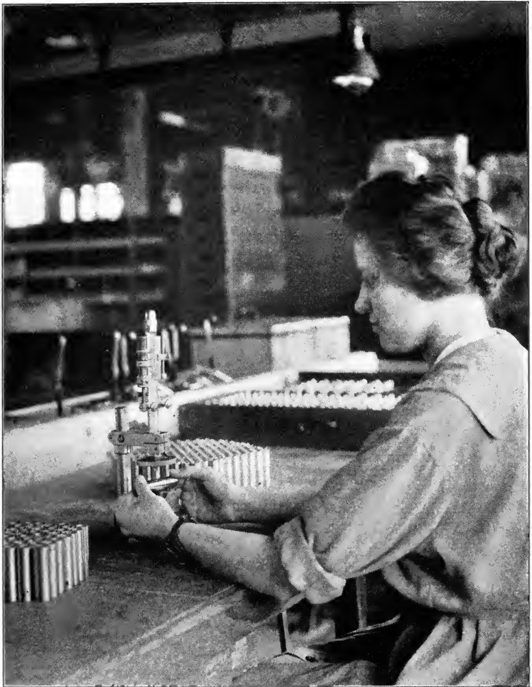
Figure 38. Prestwich Fluid Gage as Used to Inspect Piston Pins Diameter held to within 0.0002 inch—Packard Motor Car Company.
