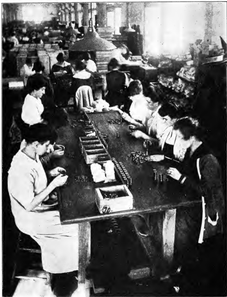
Figure 42. Inspection of Time Fuse Parts War work of American Locomotive Company.
