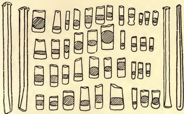
FIGURE 5. Chasing tools and punches for embossing.
