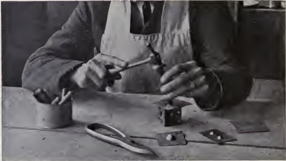
FIGURE 29. Dapping tools in use.
