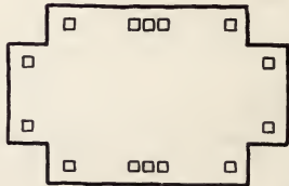
DEPRESSION MADE BY PLACING ON PITCH AND USING TOOL SHAPE OF UNIT. DEPRESSION FILLED WITH ENAMEL.
