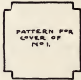
DEPRESSION MADE BY PLACING ON PITCH AND USING TOOL SHAPE OF UNIT. DEPRESSION FILLED WITH ENAMEL.
