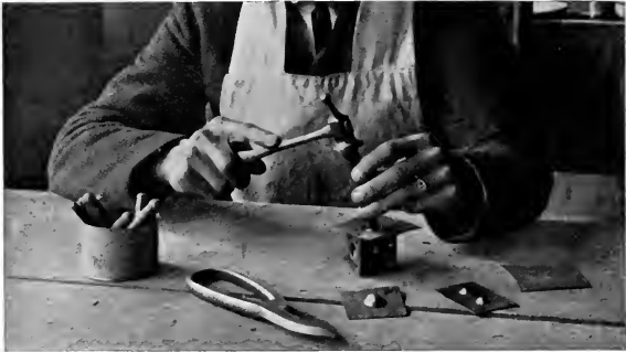
FIGURE 29. Dapping tools in use.
