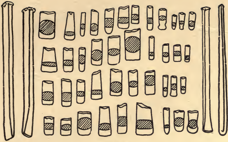
FIGURE 12. Chasing tools and punches for embossing.
