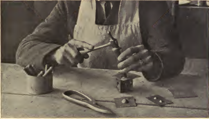
FIGURE 35. Dapping tools in use.
