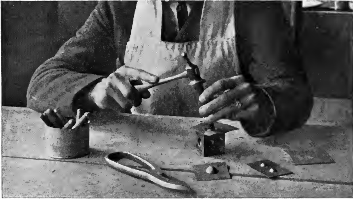
FIGURE 35. Dapping tools in use.
