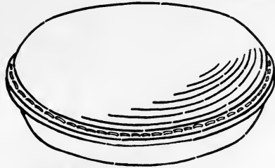
FIGURE 9. Sand bag or engraver's pad.
