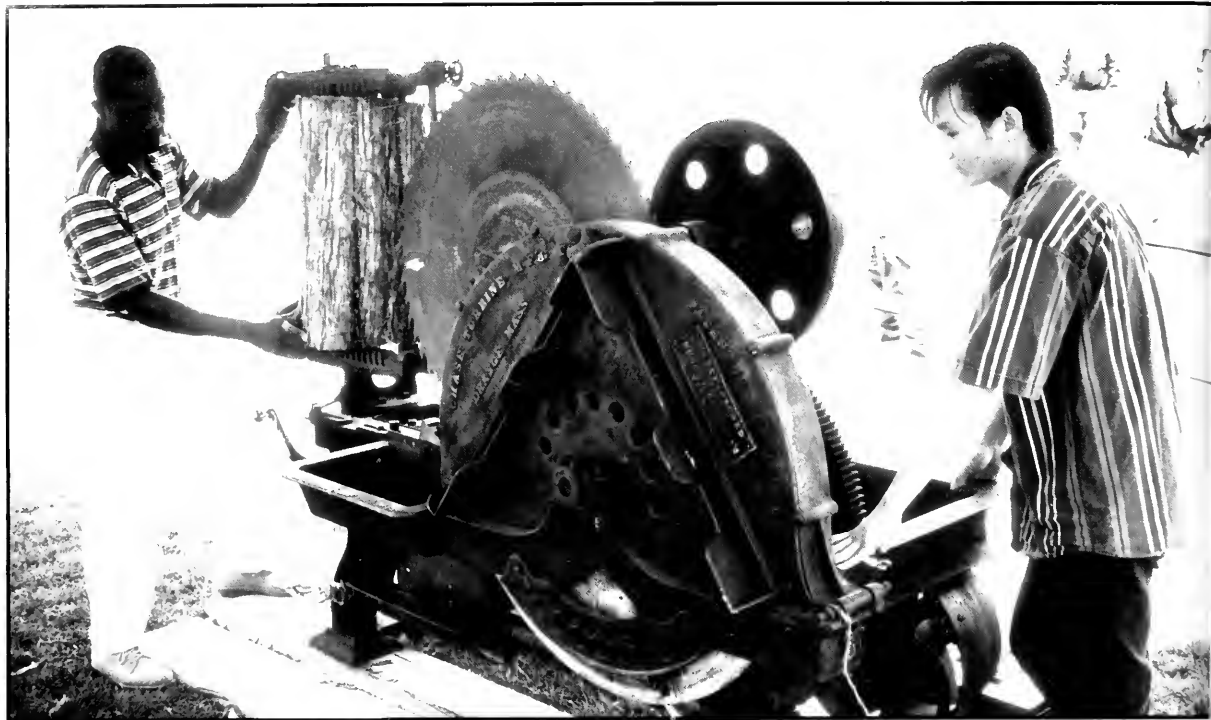
Winston Foster and Vykhua Phung To demonstrate shingle-making on a mid1800's saw.
