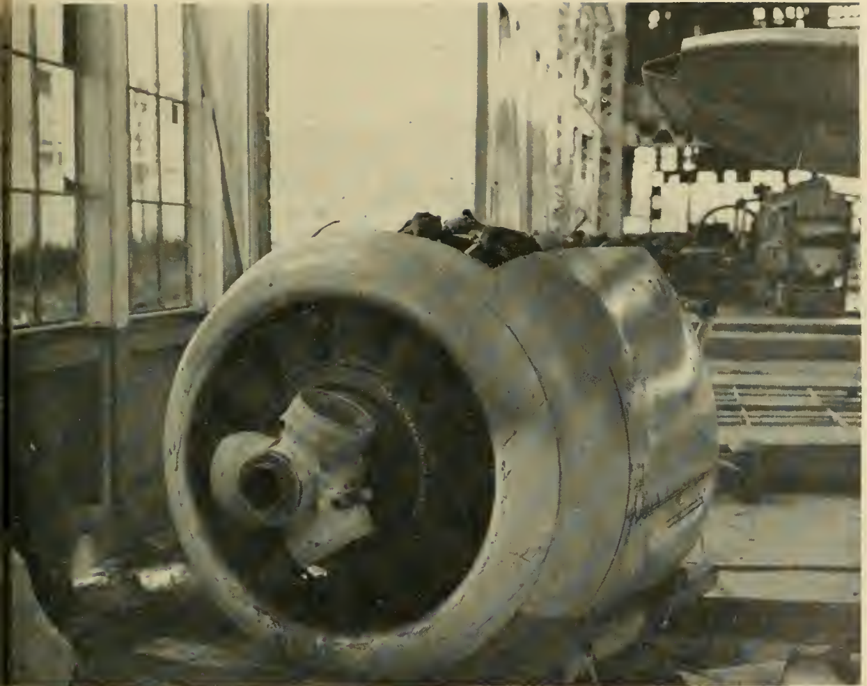
Proto No. 5.—German engine from Focke-Wulf 190 fighter found in experimental building at Kagamigahara. This was studied as model in adaptation of Tony from liquid-cooled to radial-engine installation.
