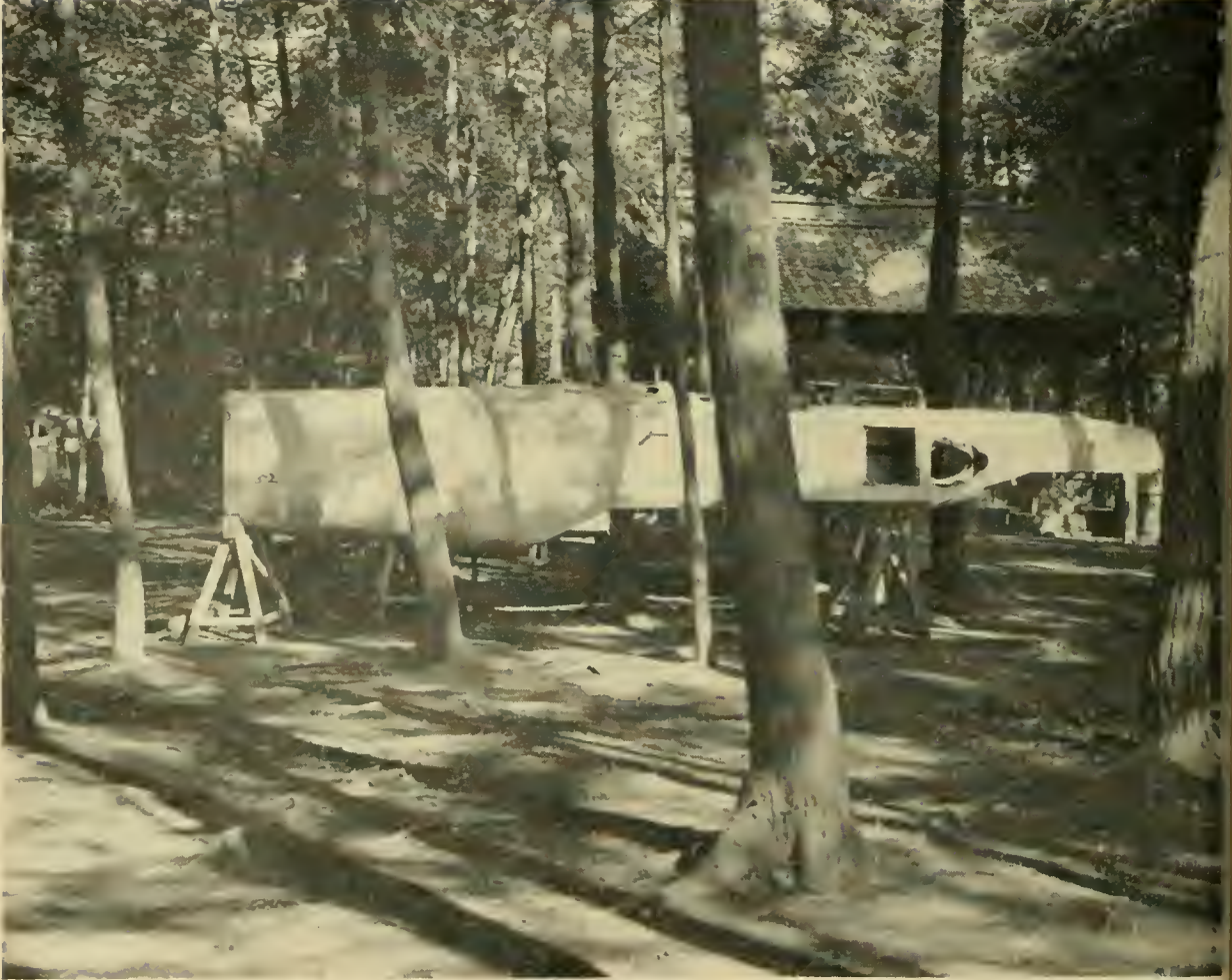
PHOTO NO. 8.—Tony fighter assemblies hidden under the trees about one half mile from Kagami-gahara works. This was part of dispersion plan which intended to use main works only as assembly shop for part of output after J raids.
