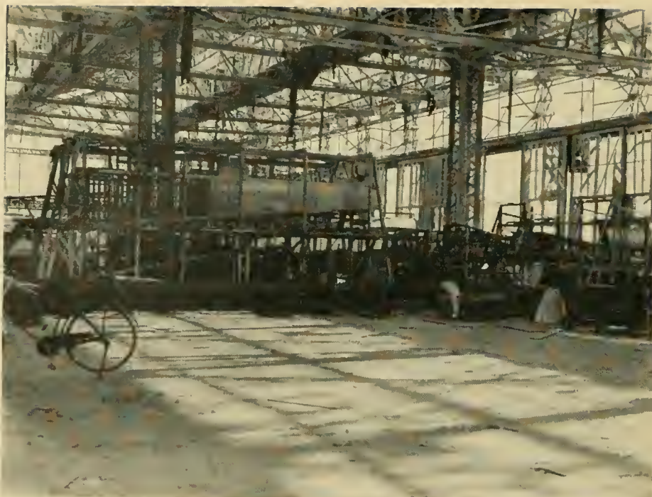
Photo No. 1.—Outer wing panel assembly jigs, Kagamigahara plant. As can be seen, jigs were light in construction but adequate.
