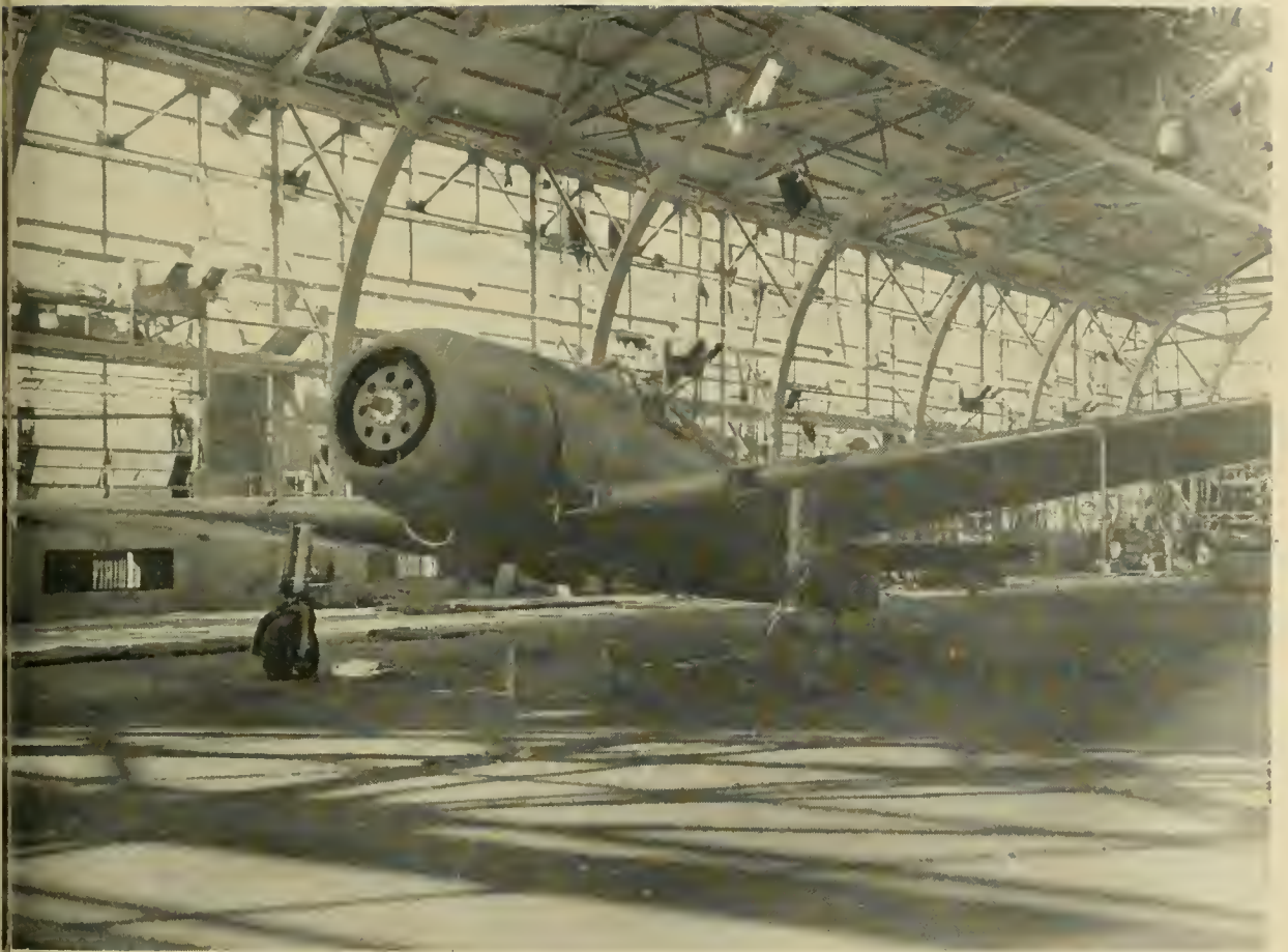
Photo No. 3.—Tony, in new radial engine version shown in final assembly building at Kagamigahara. Large arched-roof hangar-type buildings constituted about one-half of the plant's structures.
