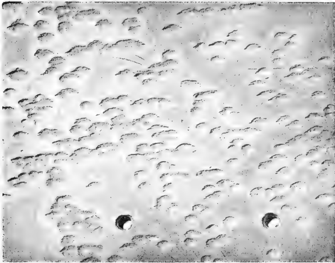
Figure 6. Pitting corrosion of nickel-copper alloy 400 after 1064 days of exposure at a depth of 5300 feet.
