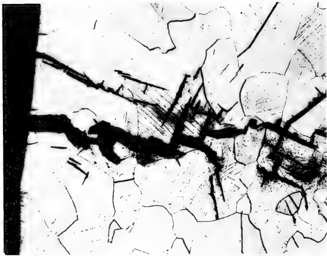
Figure 6. Secondary crack in parent metal away from and parallel to main fracture. Crack is branching in nature and transgranular. Etched in lactic, hydrofluoric and nitric acid mixture. X100.
