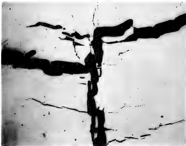
Figure 8. Irregular, branching stress corrosion crack in 13V-11Cr-3Al. Unetched. X100.
