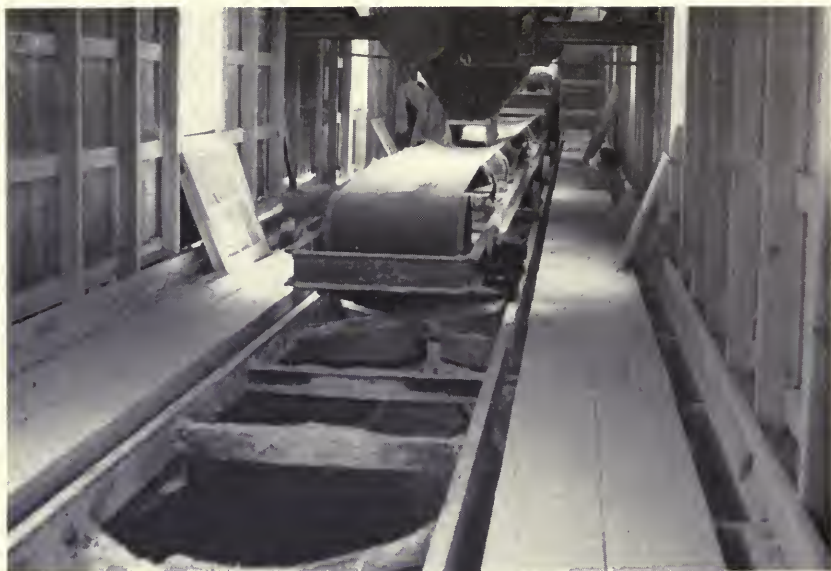
Horizontal conveyor belts, situated above the storage bins, are used in large plants to fill the bins with materials. (Fig. 10)
