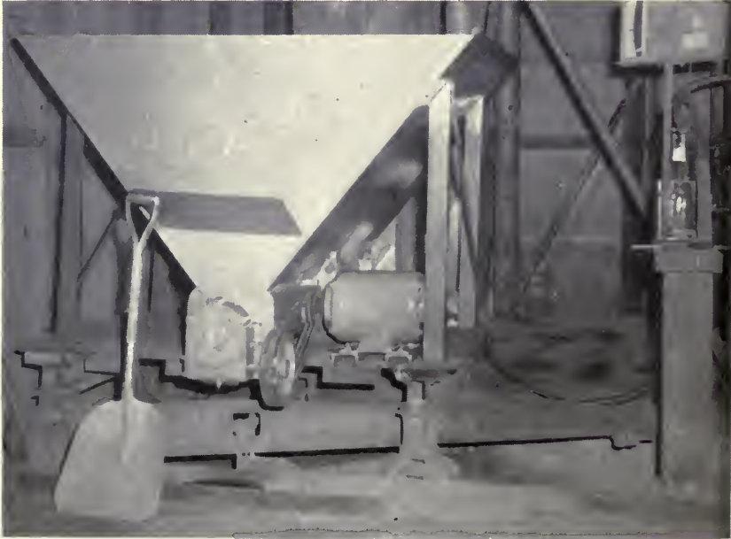
In platform scales of this type, materials are dumped into the hopper, weighed, and forced out by an auger in the bottom of the hopper. (Fig. 12)
