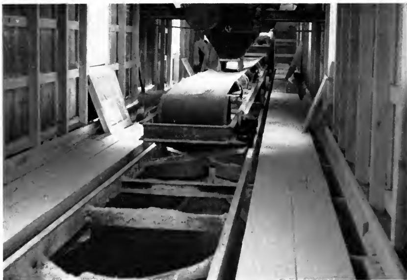
Horizontal conveyor belts, situated above the storage bins, are used in large plants to fill the bins with materials. (Fig. 10)
