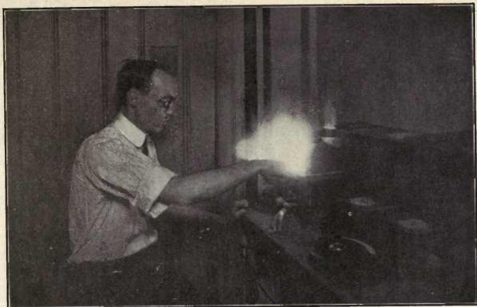
Starting a high-temperature furnace to determine the fusing point of ash in the Testing Plant of the Fuel Engineering Company. (See page 57.)
