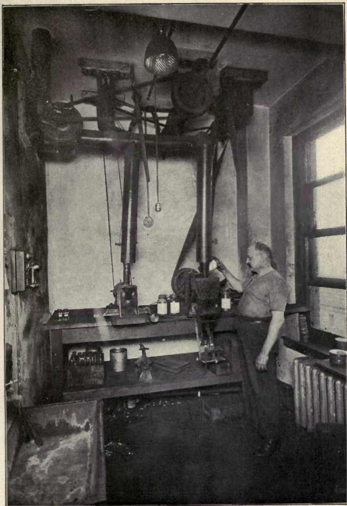
Preparation Room in the Testing Plant of the Fuel Engineering Company, where the coal samples are pulverized and automatically reduced in size for the testing.
