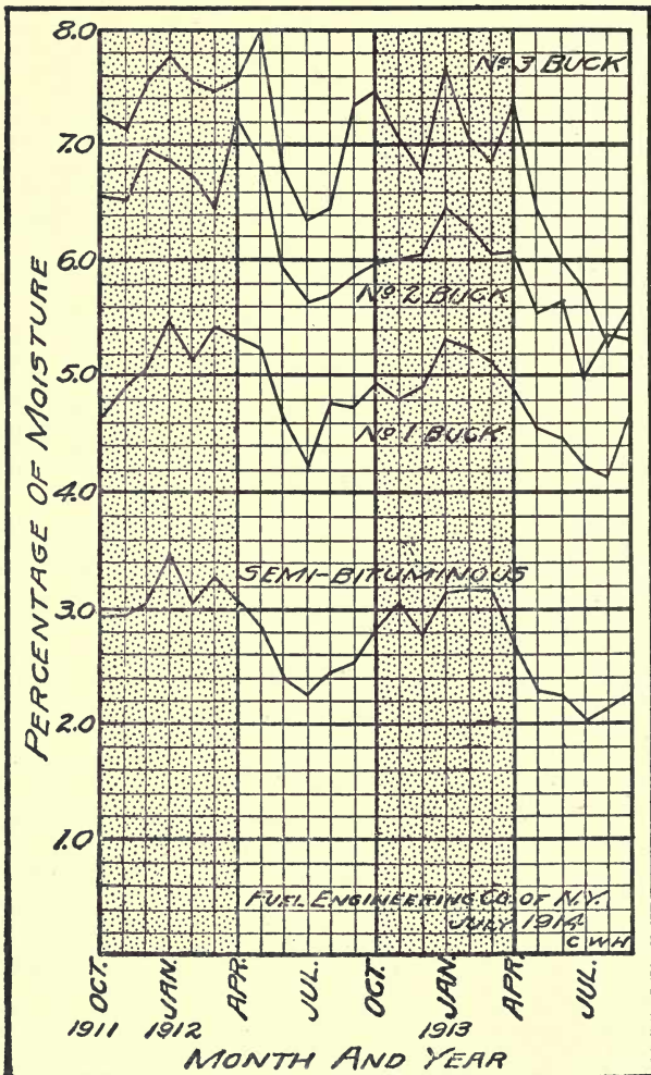
MOISTURE CHART—Notice how the amount of moisture in these four classes of coal changes in the same direction according to the season. There is a marked tendency to higher moisture during the winter months.
