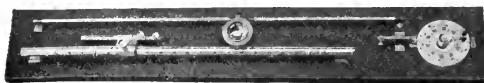
NEW TWIST TESTER WITH TAKE-UP REGISTER AND MAGNIFYING GLASS FOR SPINNING TWIST
