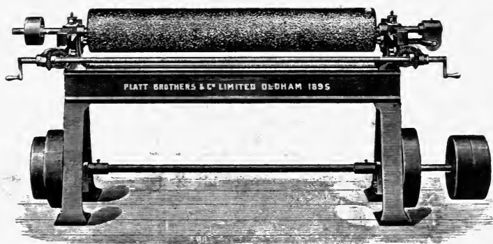
FIG. 43B.—Grinding Frame and Grinding Roller for the Rollers of Cotton Waste Cards.
