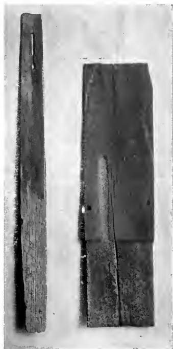
Showing differences in the wearing qualities between the hand-shaved pine and the sawed cedar shingles. The former, which is 18 \frac{1}{2} inches long, has done duty for 125 years, the latter for 15 years
