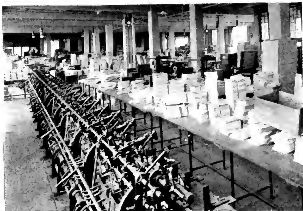
THE MACHINE THAT ASSEMBLES SUCCESSIVE PARTS OF MAGAZINE OR BOOK IN ORDER
