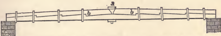
FIG. 64—Represents a solid built beam, the top part being of two pieces, b , b , which abut against a broad flat iron bolt, a , termed a king-bolt .
