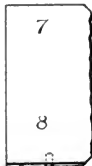
7. Sawed off 3/8" outside of knife line 8. Chamfer corner opposite working edge and plane to knife line. (Square with face and working edge.)
