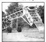
Photo shows how mainframe folds for screen maintenance.
