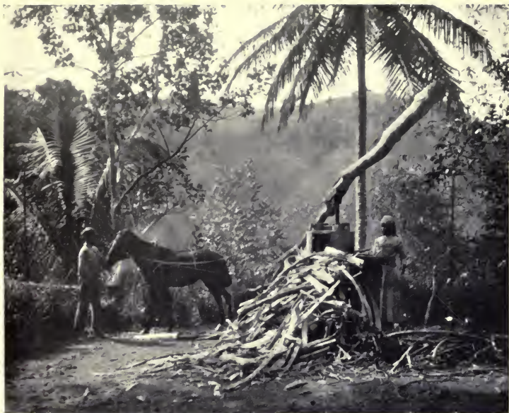
PEASANT'S PRIMITIVE SUGAR-GRINDING MILL
