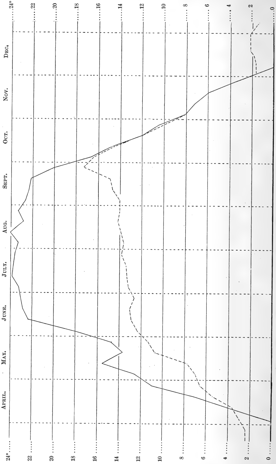
FIG. 1.—Surface and bottom (18 m) temperatures, 1895. Full line, surface; broken line, bottom.
