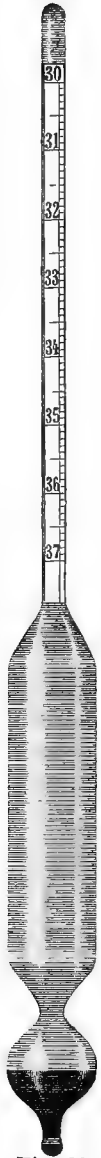
Fig. 32. Beaumé hy- drometer for sweetened condensed milk Courtesy C. J. Tagliabue Mfg. Co.
