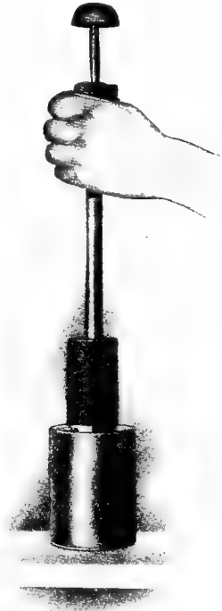
Fig. 45. A convenient device for soldering by hand
