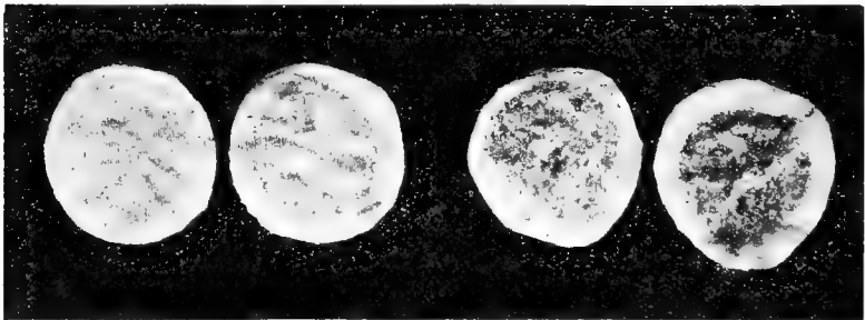
Fig. 10. Cotton Filters Clean milk Dirty milk
