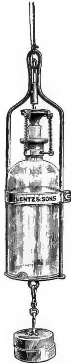
FIG. 60. — Apparatus for collecting water samples (after Abbott).
