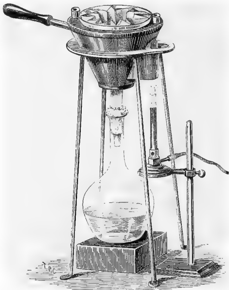
FIG. 6.—HOT-WATER FILTER FOR FILTERING NUTRITIVE GELATINE OR AGAR-AGAR MIXTURE.
