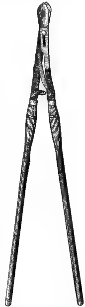
FIG. 79. — Tool for taking out the old canes that have borne fruit one season.
