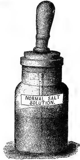
FIG. 129.—DROPPING-BOTTLE OILER, WITH DROPPING TUBE REMOVED; x.5.
