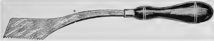
FIG. 144.—SMITH'S SIDE-BONE SAW (EARLY PATTERN).
