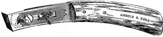
FIG. 66.—THE SPECIAL DRAWING-KNIFE (FLEMING'S) FOR PREPARING THE FOOT FOR THE CHARLIER SHOE.
