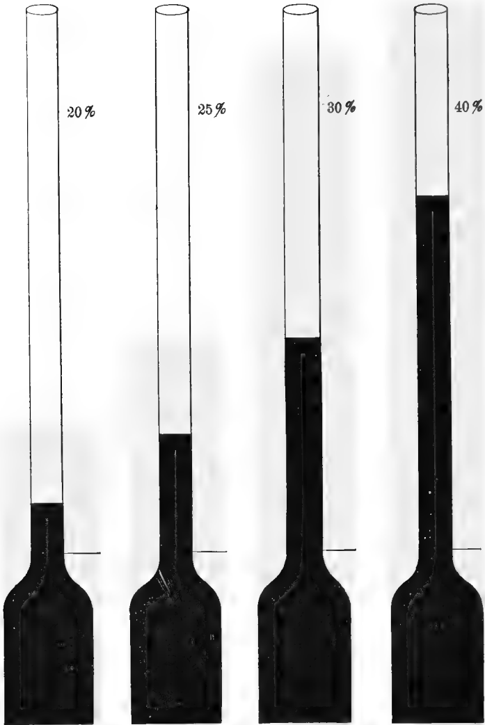
FIG. 91.—Showing the height to which cream free from air-bubbles must be raised in a pipette to get 18 grams of cream. It shows that to measure cream in a pipette is inaccurate in cream testing. (Iowa State Dairy Com. Report, 1903.)
