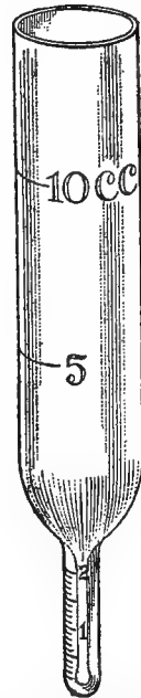
FIG. 39.—Sediment tube used in the Trommsdorff test, showing graduations in the capillary extension at the bottom.
