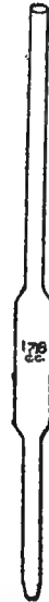
FIG. 34.—Pipette used in Babcock test for measuring milk. (From Chemical Testing of Milk and Cream , by R. H. Shaw, U. S. Dept. of Agriculture.)
