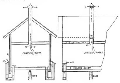
Fig. 58.—The Rutherford System of Ventilation.
