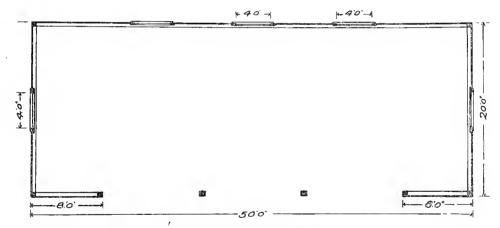
Fig. 60.-Floor Plan of Shed.
